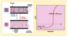
Thus the polyfuse acts like a self-resetting solid-state circuit breaker, which makes it suitable for providing low cost over protection. The resistance of polyfuse at room temperature is in the order of few ohms.
